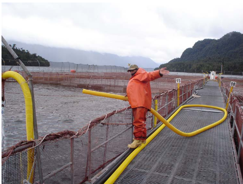
Photo 16. Fish farm worker feeding with semi-automatic system.
